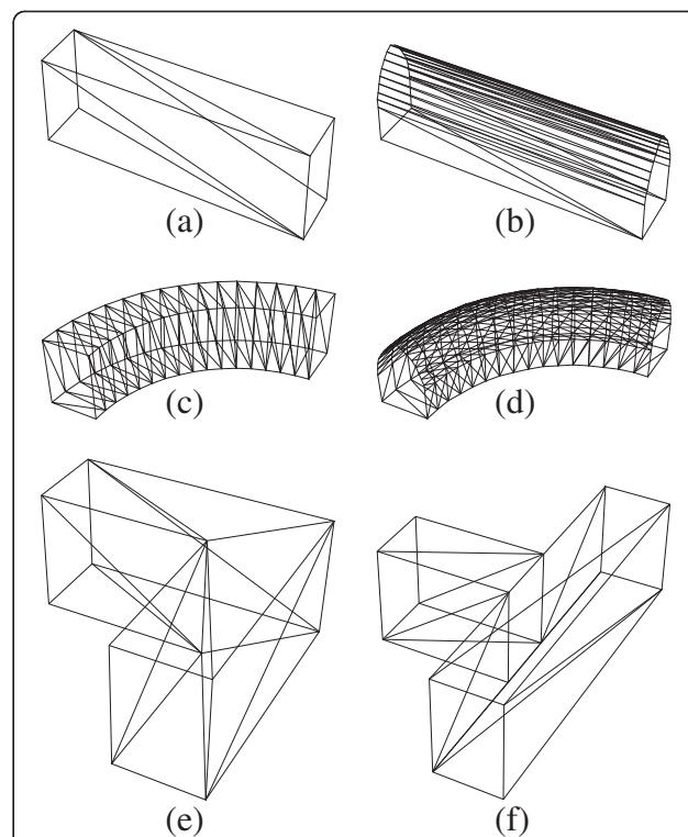
**Figure 4** A straight shape corridor with (a) rectangular cross section modeled by triangular facets, (b) arched cross section modeled by triangular facets. A curved shape corridor with (c) rectangular cross section modeled by triangular facets, (d) arched cross section modeled by triangular facets. (e) A L-shape corridor with rectangular cross section modeled by triangular facets. (f) A T-shape corridor with rectangular cross section modeled by triangular facets.
