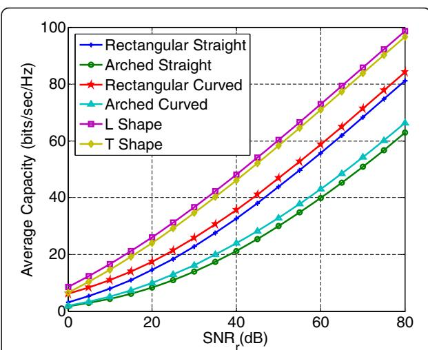
**Figure 10** Capacity versus  $\text{SNR}_r$  for the six different geometrical configurations of corridors.
