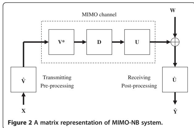
**Figure 2** A matrix representation of MIMO-NB system.
