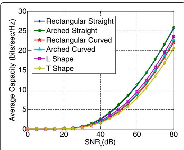
**Figure 9** Capacity versus  $\text{SNR}_t$  for the six different geometrical configurations of corridors.
