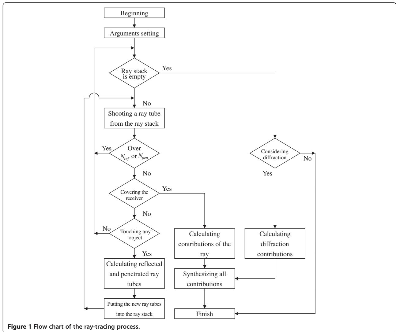
**Figure 1** Flow chart of the ray-tracing process.
